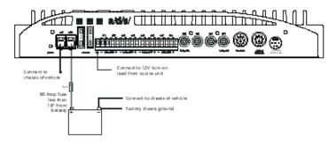
speaker connections for stereo configurations
